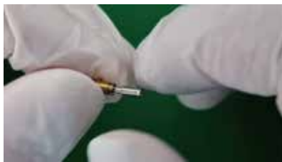
将螺丝拧入SFIT®Ti-Base
